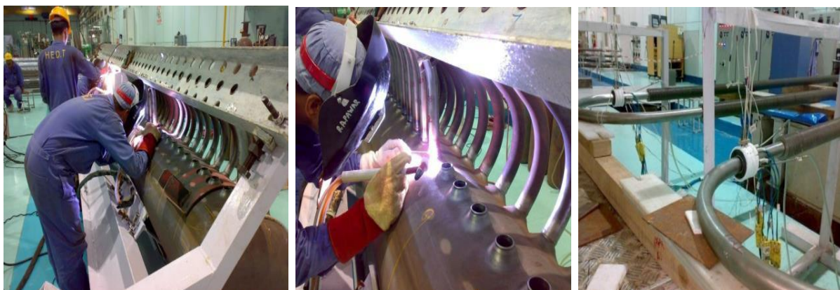
Fig.7: Tube bundle fabrication of AHX- A.
