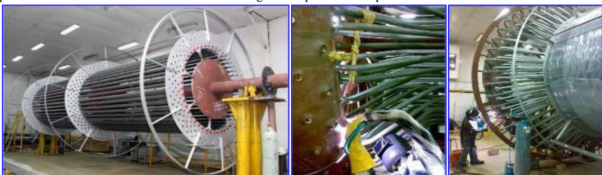
Fig.6: Tube bundle fabrication of AHX- B.
